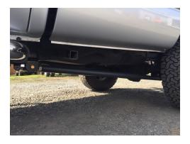
Tighten jamnut and all hardware fully. Check all hardware after 100 miles.
