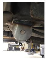
Weld brackets on a minimum of 3 sides, paint, and fully install bars.
