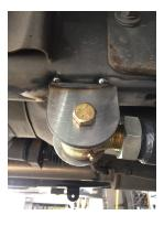
Bolt bars into desired length and prep are frame where brackets will land. Then tack brackets into place.
