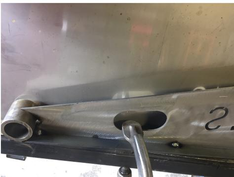
Clamping helps to flatten out areas of the flatbar. Do this to other side and weld out with 1" welds.
