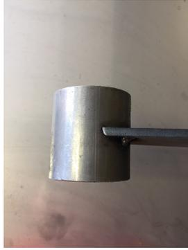
Tack 2" tube centered on axle end of bar.
